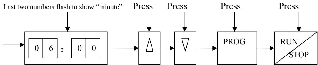
3. Soft start: The RPM starts from “0” and reaches to the set speed in 30 seconds. It shows time and speed alternately during running.
