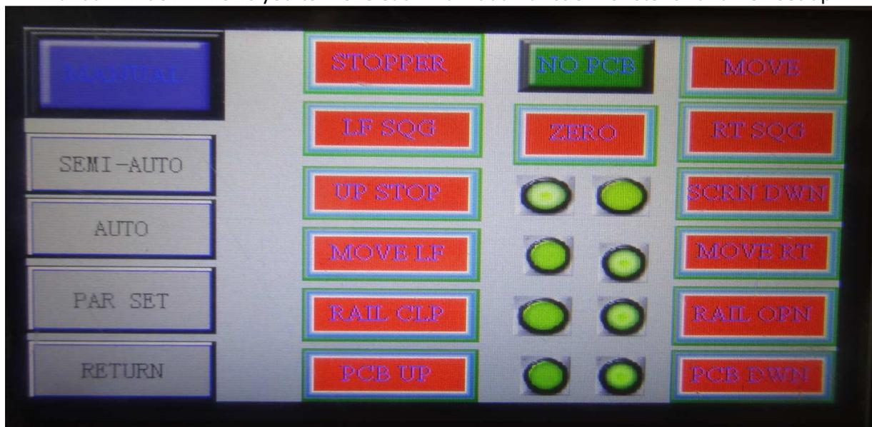
Stopper: UP/Down PCB stopping point location.
