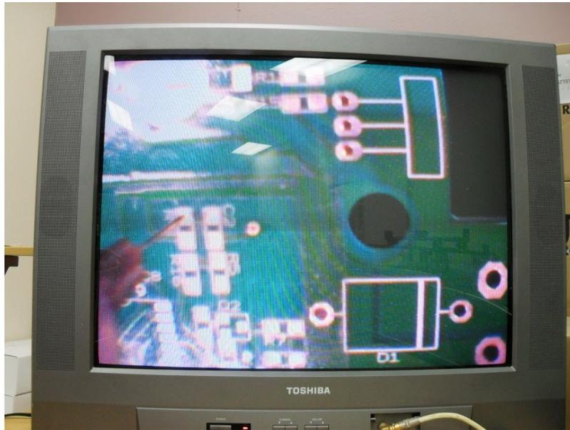
2. Look at the circuit board and check if the needle moves to corresponding position. Because the camera is not straight and the needle may be a little bit bend, the real location you want to dispense is not the position you see on the monitor. Adjust the needle manually and at the same time check the circuit board to make sure that the needle is at the center of the item you want to dispense. The current position can be set as X2, Y2.
