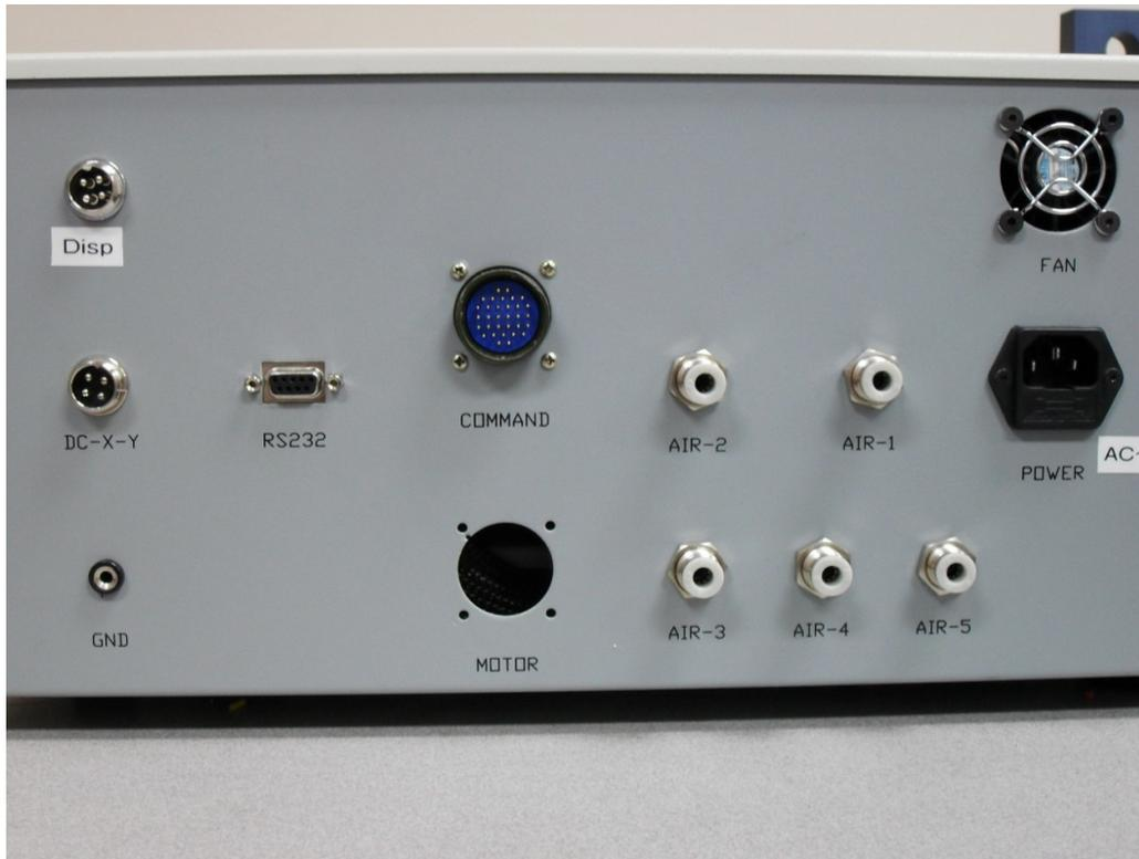
Back of the machine control box
